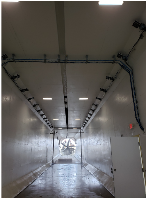
Figure 6: Test section of WVU Free-Flight Wind-Tunnel that is outfitted with a 40 camera VICON motion capture system.
